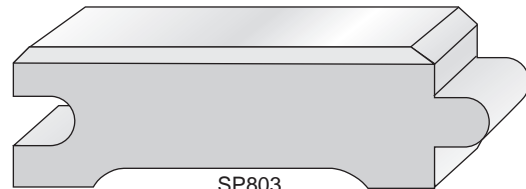
SP803 Flooring with small "v" groove 3/4" X 2 1/2" to 6"
